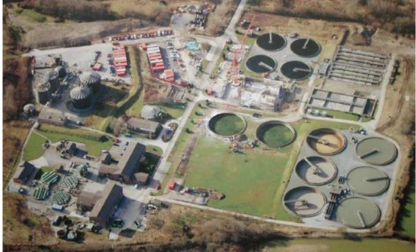
The old treatment works in Llanelli and Gowerton were converted into pumping stations and the flows transferred to the new works. The existing CSOs were improved with screening and some of the sites were also provided with storage in order to reduce the number of spills to the environment.
