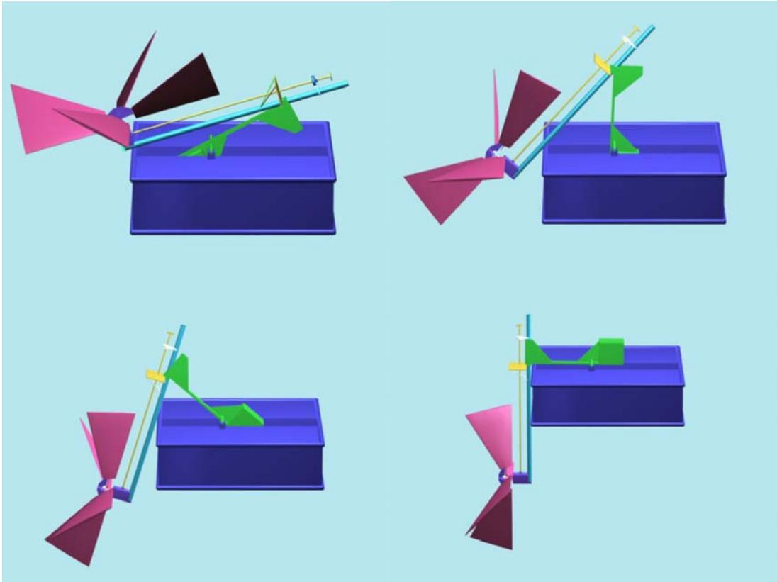
Deployment of turbine hub-leg assembly
