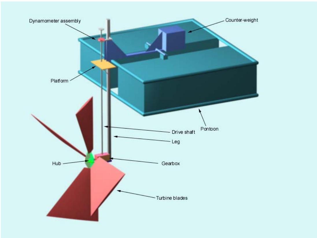
General arrangement of pontoon, leg and turbine on test rig
