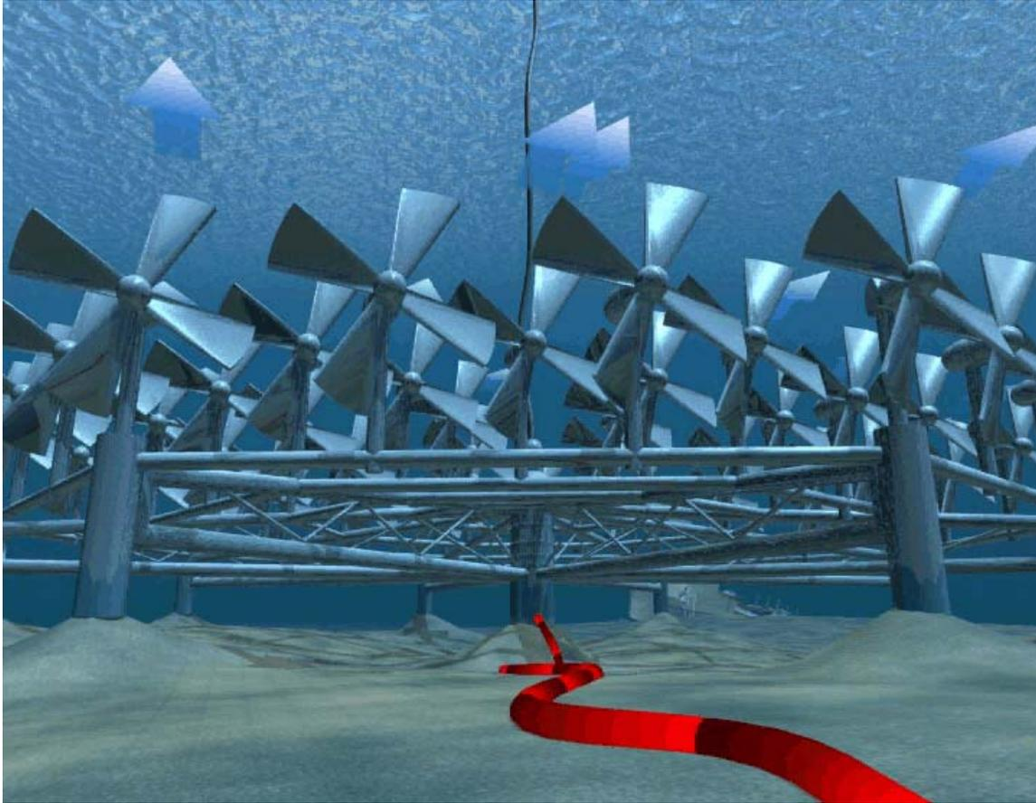
**TYPICAL SEABED INSTALLATION. THE UNIT IS BALLASTED TO HOLD IN PLACE. THE TURBINE HEADS CAN TURN THROUGH 360 DEGREES TO SEEK THE TIDAL DIRECTION. THE ABOVE IS SCHEMATIC ONLY, AND DOES NOT SHOW THE ACTUAL BLADE SHAPE , CLEANING SYSTEM, BEARING SYSTEM ETC.**
