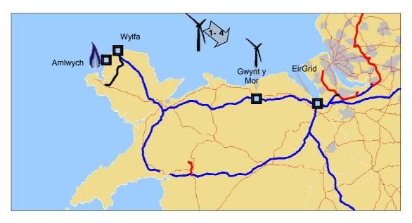
Blue lines represent the National Grid 400kV system and the red lines represent the 275kV system.
