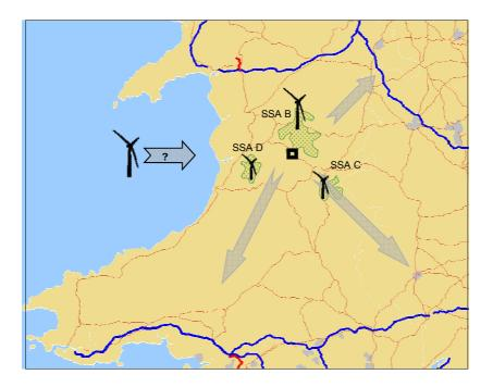
Blue lines represent the National Grid 400kV system and the red lines represent the 275kV system.
