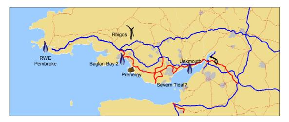
Blue lines represent the National Grid 400kV system and the red lines represent the 275kV system.
